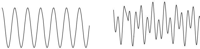
Fig. 11.1.1. Realizations of Gaussian sample paths with the spectrum (11.1.7) and second spectral moments \lambda_2 = 200 (left) and \lambda_2 = 1,000 (right).
